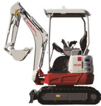
1.6 t Excavator/w trailer
